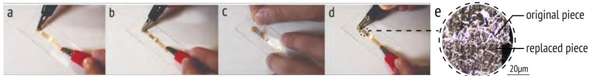
Fig. 5. (a) Silver trace is transferred onto PDMS and connected with LED. (b) Part of the trace is removed. (c) Recovering the damaged portion with a new silver trace. (d) The silver trace is recovered. (e) Microscopic image of the edge between the original and the replaced silver trace.
