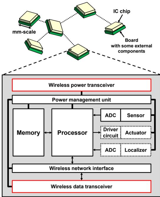
**Figure 2.** Architecture of computing particles.
