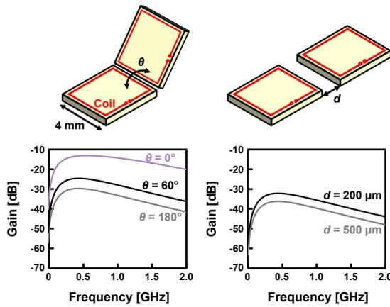
**Figure 3.** Magnetic coupling characteristics of on-chip antennas.
