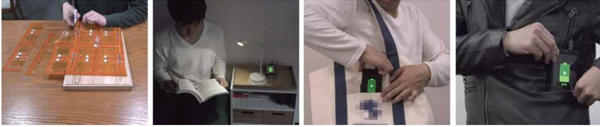
Fig. 1. Our cuttable WPT sheet allows the fabrication of WPT surfaces through a simple physical “cut-and-paste” process. We introduce three application examples: wireless charging shelf, bag, and jacket.
