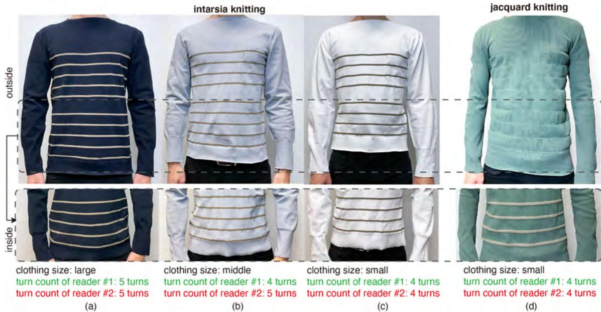
Fig. 6. Four prototypes of our textile-based reader coil knitted using (a)–(c) intarsia technique and (d) jacquard technique.
