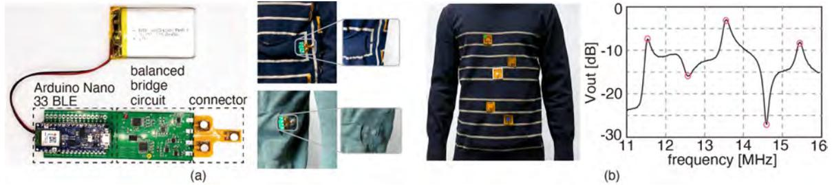
Fig. 9. (a) Overview of our impedance measurement module. The module is connected to the clothing via the magnetic connector. (b) Example of signal processing when five different sensor coils are placed on the clothing. Based on the output values, the PC detects the frequency peaks based on a peak detection algorithm, and then, calculates the peak shift.
