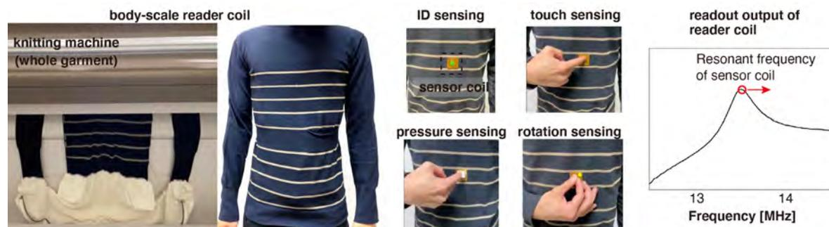
Fig. 1. Twin Meander Coil is fabricated on garments using industrial knitting machines and can wirelessly read out on-body battery-free sensors placed throughout the garment surface.
